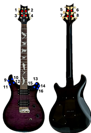
Figure 4: PhaseSpace guitar markers' placement. On the left is the front view of the guitar, and on the right is the back view. Four markers (1–4) were placed on the front of the head, four on the back of the head (5–8), and eight markers on the body (9–15).
