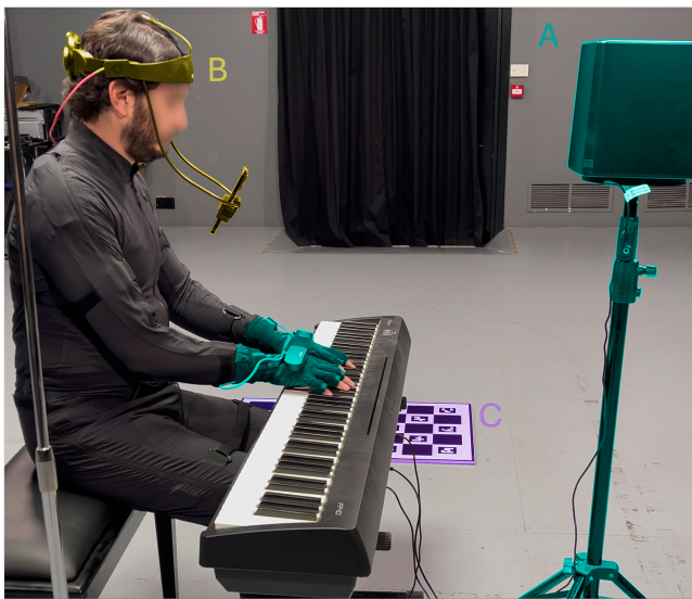
Figure 2: The musician, dressed in a Rokoko MoCap suit, performs on a digital piano. "A" shows the coil pro (the right box in the tripod), used with the gloves to enable accurate finger capture. "B" shows the headrig used for capturing facial data with an iPhone. "C" displays the ChArUco board placed on the floor to facilitate camera parameter calibration.
