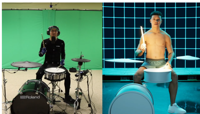
Figure 5: Use of a motion capture system to holistically track a musician (full-body, face, fingers), drum sticks, and drums. Image extracted from [Cin21].
