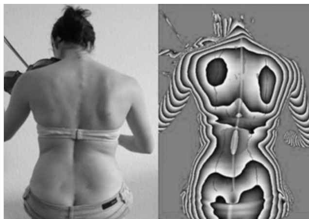
Figure 7: Analysis of the upper body posture of a musician playing high-stringed bow instrument using 3D back scans. Image extracted from [OMB*18].
